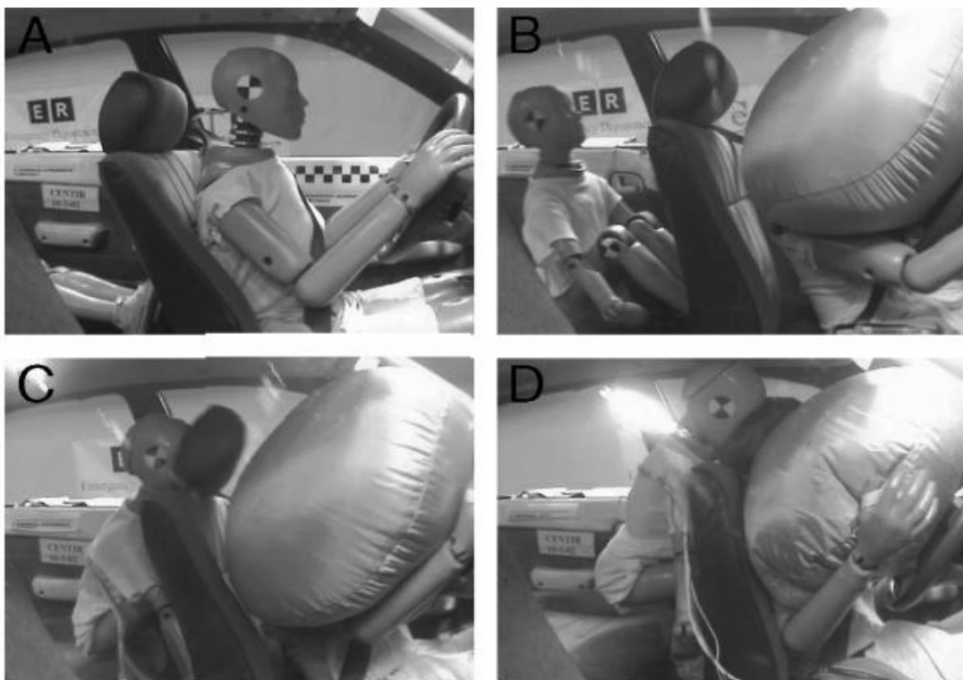
Figure 3. Six Year Old Unbelted Child in Rear Seat Strikes Belted Driver in Sled Test.
