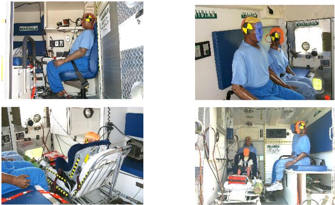
Figure 4. Location of Anthropometric Test Dummies (ATDs) within the test vehicles.
